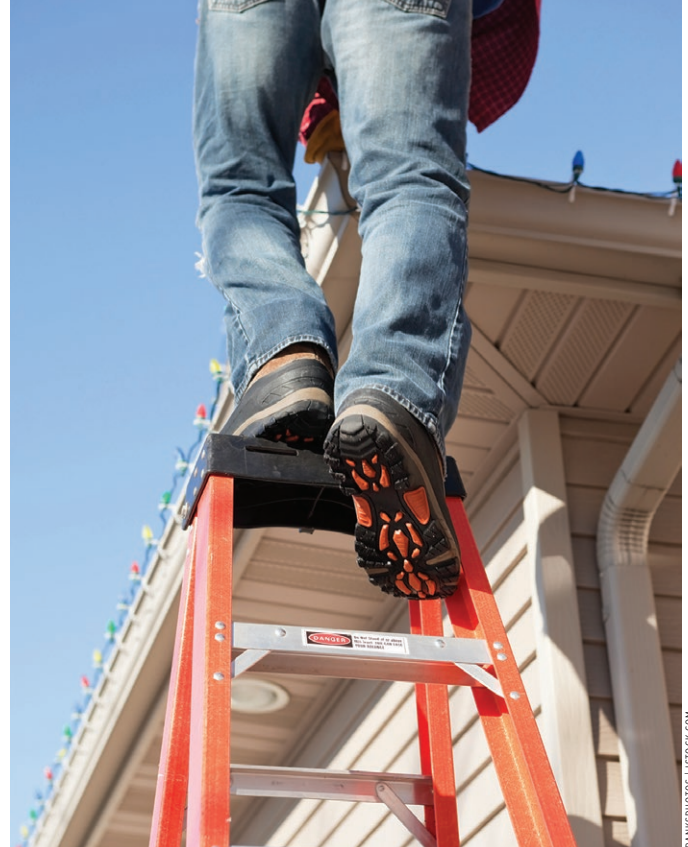
Stepping to the very top of a ladder is a no-no, as the warning label clearly indicates.
